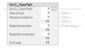
Motion Axis Gear configures a Slave Axis to be electronically geared to a Master Axis with a specified ratio. The ratio is defined in using a Ratio and Denominator.
