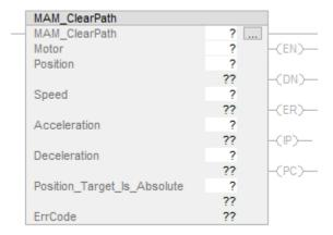
Motion Axis Move commands the servo to move to a specified position. The positional move will execute on the servo each time the rung-condition-in transitions from FALSE to TRUE.
